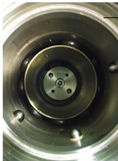
Installed Metal O-ring
